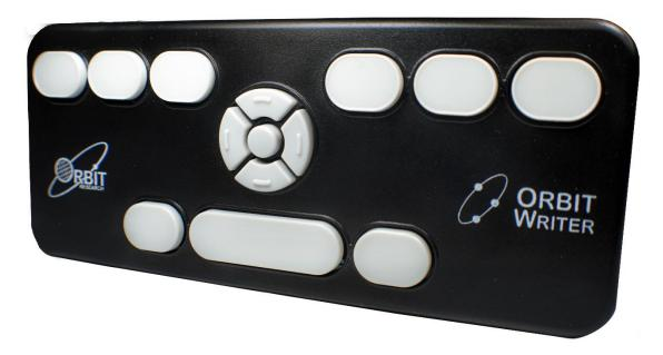
The Orbit Writer is a compact and portable Perkins-style braille keypad with the following features.
